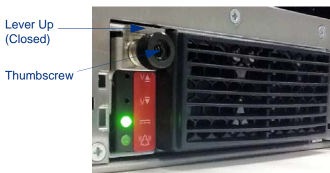
Figure 28. AC Power Supply Unit: Ejector/Insertion Lever (Close)
