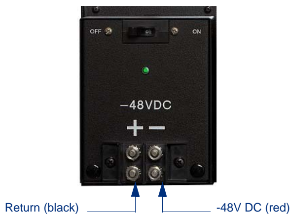
Figure 25. DC PEM Cable Connectors
