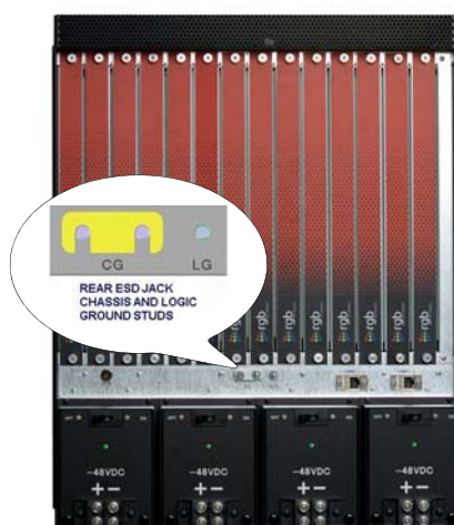
Figure 24. Chassis (rear) Ground and Logic Ground—DC System
