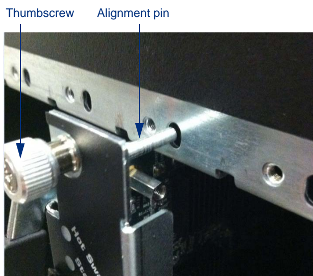
Figure 23. Card insertion—alignment
