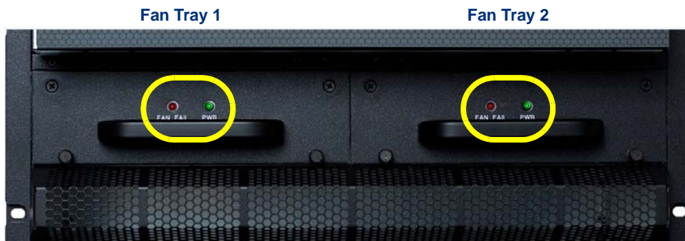
Figure 10. Fan Tray LEDs
